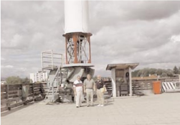
Antenna mounted on turntable for HRP measurement. Ray Carnovale, Greg James, Dirk Freeman.
